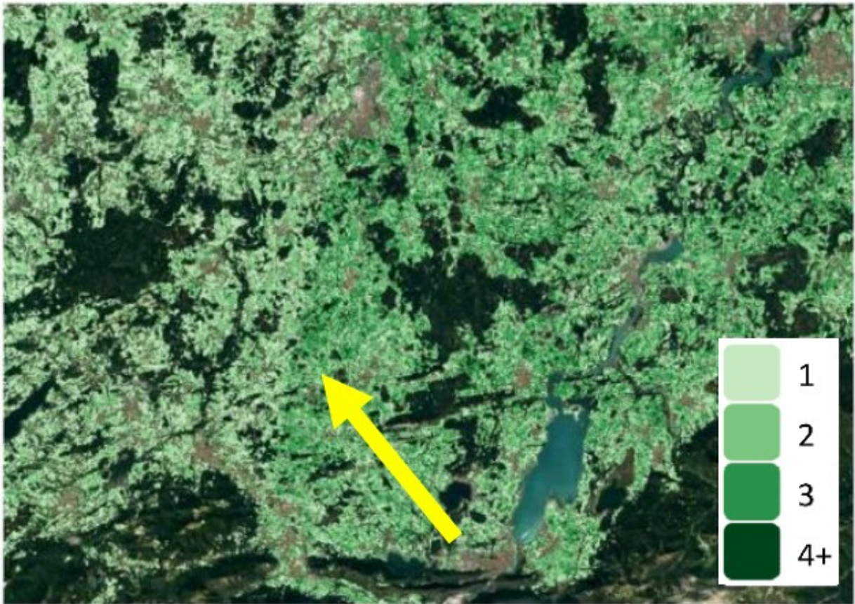
Figure 17: Visibility of the Sentinel-2 swath borders and the different swath coverage in the GRAME layer (32TPT; WGS84 coordinates: 10.63480°E, 47.65318°N).
