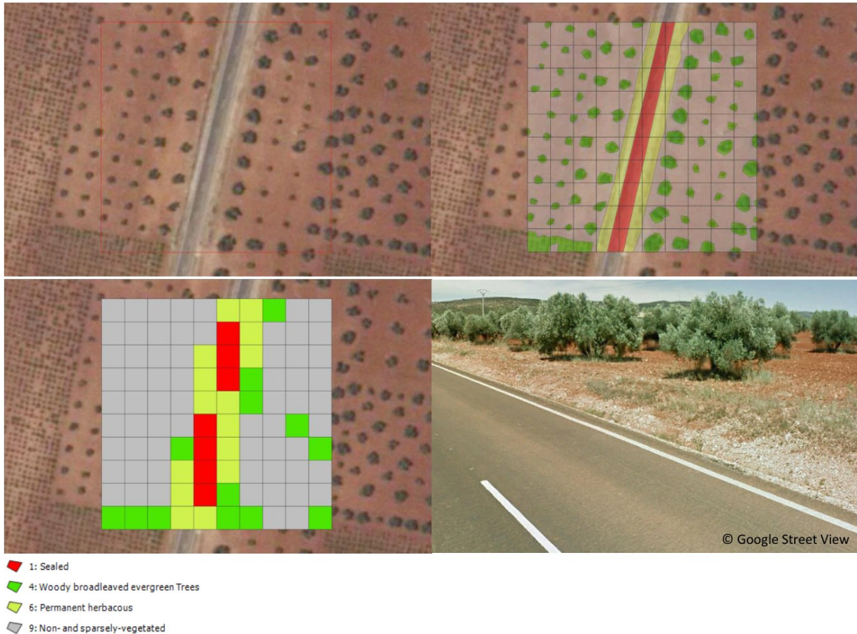
Figure 6: Illustration of the CLC+ Backbone Raster Product decision tree approach to evaluate area thresholds for mixed land cover at olive groves, Castile-La Mancha, Spain. Upper left: 100x100m plot overlaid on aerial imagery. Upper right: Outlines of surfaces which are covered by Sealed, Permanent herbaceous, Broadleaved evergreen trees and Non- and sparsely-vegetated. 10m pixel grid overlaid on top. Lower left: Resulting class attribution of the 10m pixels when applying the threshold of Biotic >30% to decide between Non- and sparsely-vegetated vs. one of the vegetation classes. Lower right: ©Google Street View of the area, showing the four dominant land cover classes.
