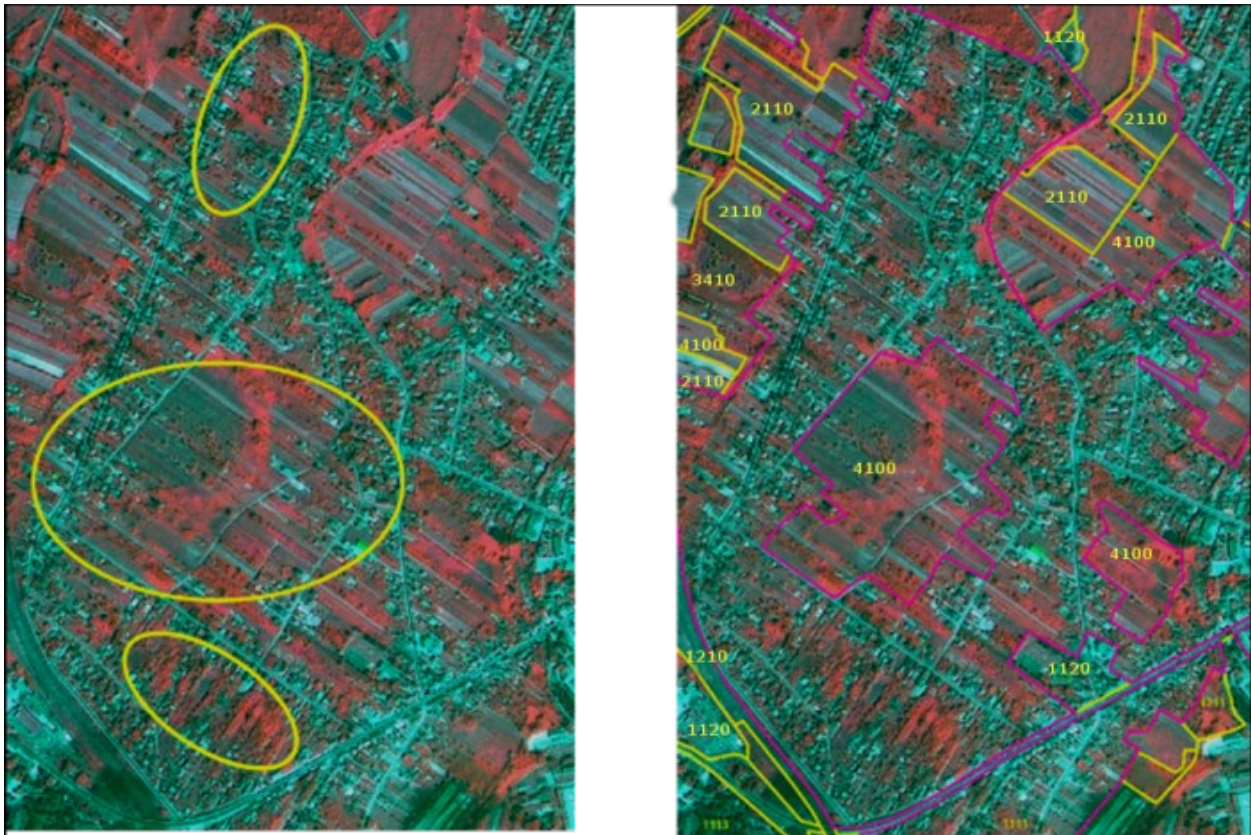
Generalize urban outline, include gardens, and use class 2.3.2.0 for complex areas (example from Poland). SPOT-5 (2.5m) (Poland) (1/2/3 Band Combination). Date: 2011-07-23. Source: CNES 2011©, Distribution Airbus DS/Spot Image
