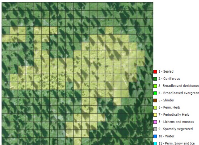
Figure 8: CLC+ BB Raster Product superimposed on ESRI World Imagery (left) and VHR IMAGE 2021 (right) for an area with sparse tree cover in the Alps. Sparse tree canopies dominated by herbaceous understory are mapped largely correct as class 6.
